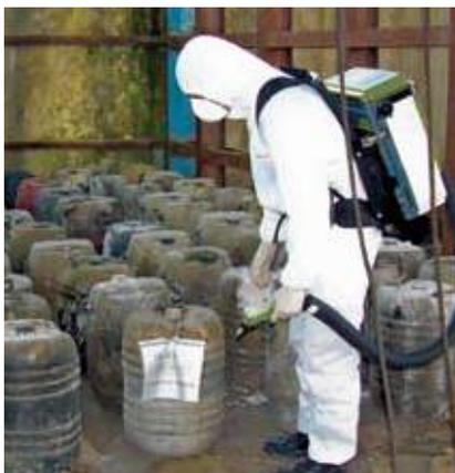
HAPSITE ER has the capability to identify analytes in the PPM (parts per million) – PPT (parts per trillion) range. The GC column provides sharp chromatography and excellent resolution. During the quantitation method, the front panel clearly displays what chemicals are present, their concentration, and access to information regarding the degree of danger — to help make quick decisions affecting life, health and safety.
